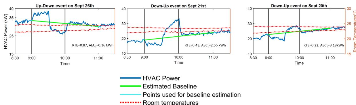
Figure 7. Three representative events at the Rackham Building including HVAC power consumption (left axis) and room temperatures (right axis).
