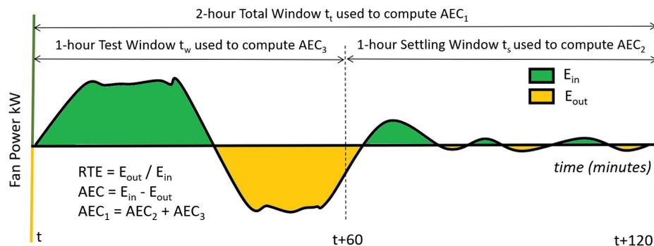
Figure 3. Metrics used to quantify the building response efficiency, where  $E_{in}$  and  $E_{out}$  are both defined as positive.
