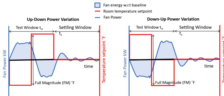
Figure 1. Up-Down (left) and Down-Up (right) power variation resulting from temperature setpoint changes.
