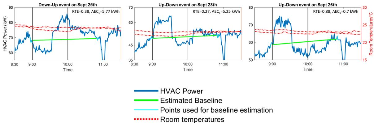
Figure 6. Three representative events at Weill Hall including HVAC power consumption (left axis) and room temperatures (right axis).
